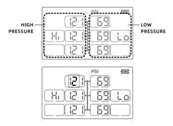
Press the **"CODE"** button to set the third number while it is flashing. After setting the pressure parameter, repeat Step 3 to set the HIGH & LOW PRESSURE ALERT parameter for all the truck axle.
