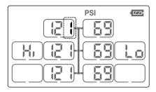
**Step 4:** After setting the HIGH&LOW PRESSURE ALERT parameter of each truck axle, shortly press the **"SET"** button to set the HIGH&LOW PRESSURE ALERT parameter of T1 trailer and the tire pressure value second number will flash. Shortly press the **"+"** or **"-"** button to set the desired pressure.
