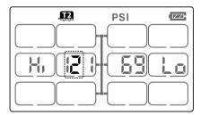
Press the **"CODE"** button to set the next number while it is flashing. After setting the pressure parameter, repeat Step 4 to set the HIGH & LOW PRESSURE ALERT parameter for T2, T3 truck. Long press the **"SET"** button to save the above operation and return to the **Standby** mode.
