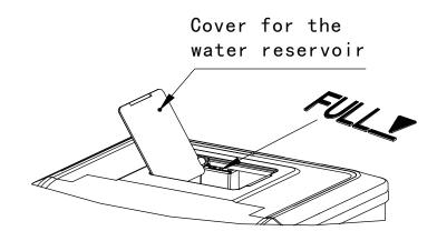
Warning: Do not pour the water into the internal water tank located underneath the ice basket. This tank is not big enough and will effect the ice making performance.
