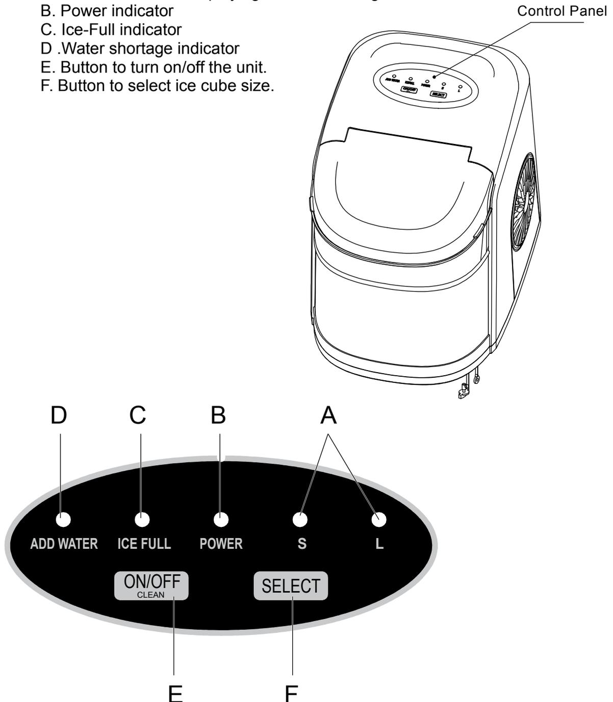
Start the self-cleaning program: Plug on the unit, then press "ON/OFF" button for more than 5 seconds to enter the self-Cleaning program. Self-cleaning program need 30 mins. When the program is over, please drain out the water and clean inside.
